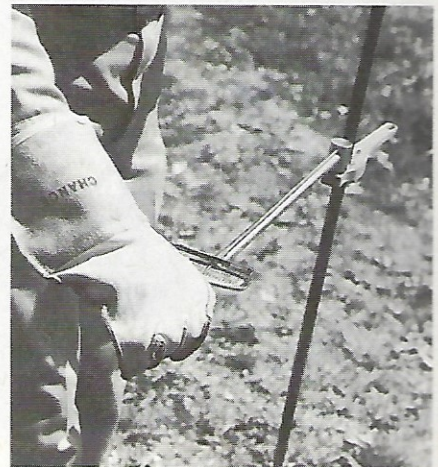
2. Test probe is driven into the ground with a calibrated torque wrench that slides up and down the square shaft
