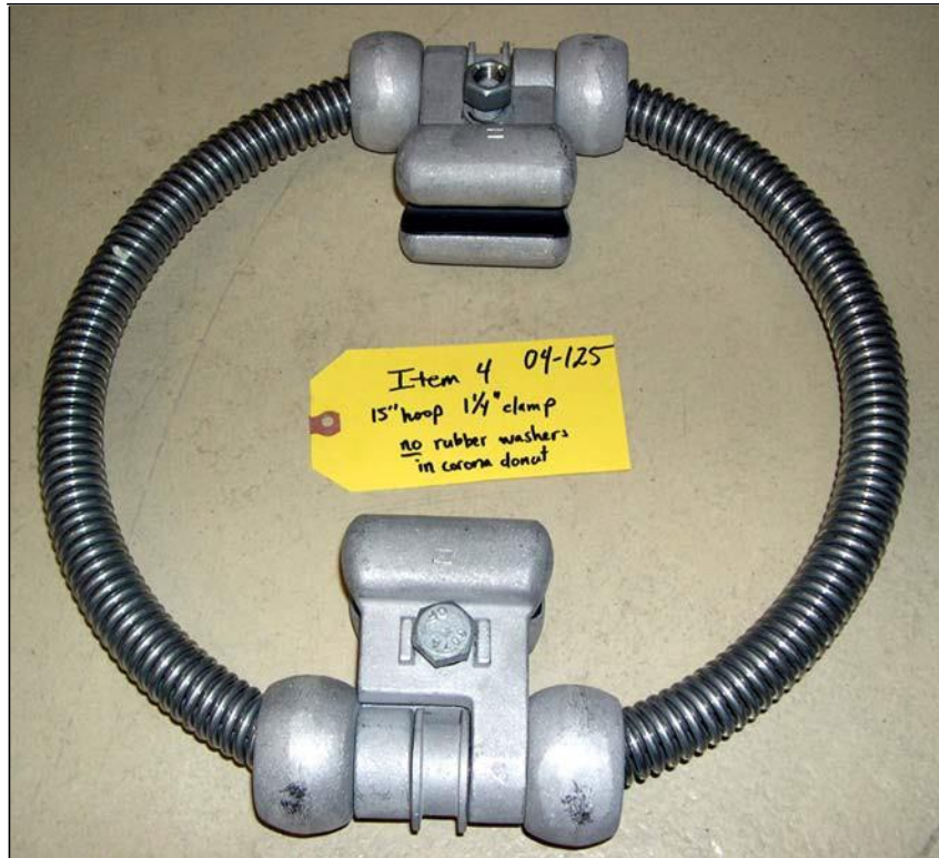
Figure 3: Item #4 Ring Spacer with insulating neoprene insert on one-half of each clamp.
