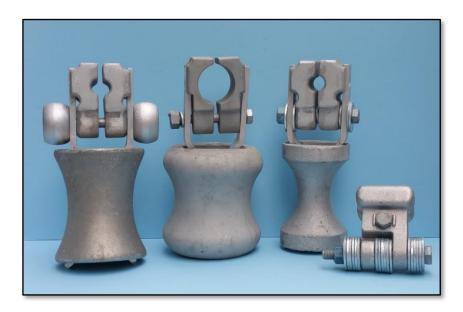
A vibration control and anti-galloping damper, this solution for shorter spans twists a single conductor, by inertia offset, both statically and dynamically. Vibration control is achieved by allowing the eccentric weight to move against the vibration. Used on power line conductors having shorter spans, it has been installed by helicopter at hot line voltages up to 161kV, and by bucket truck at voltages up to 345kV. The AR Twister has eliminated breaker operations on treated lines.
